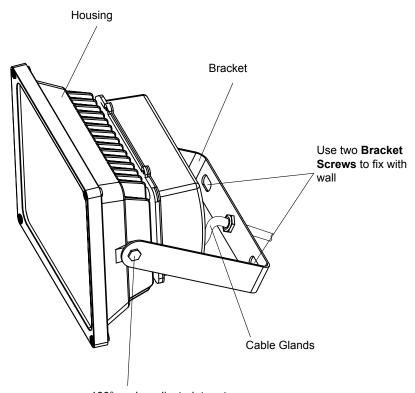
180°can be adjusted, turn two **Rotation screws** to adjusted
